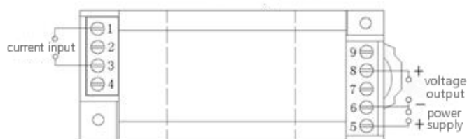
Figure 9 CE-IJ03-**MS1 Connections diagram with voltage output
