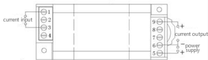
Figure8 CE-IJ03-**MS1 Connections diagram with current output
