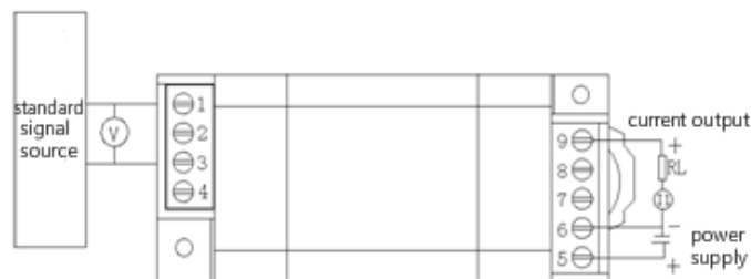
Figure 9, accuracy test wiring diagram of current output
