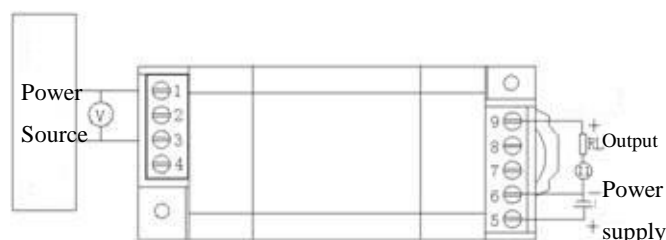
Figure 6 accuracy test wiring diagram of voltage input current
