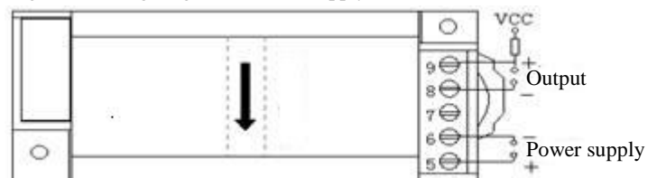
Figure 9, wiring diagram of frequency output of CE-IJ03A-F**S*
