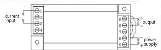
Figure 3, voltage/current output connection diagram
